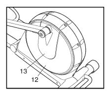
Cover (13) using a flat screwdriver. Next, remove the four Screws (not shown) from the center of the left Disc (12). Gently rotate the Disc Cover and the Disc away from the elliptical exerciser.
