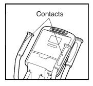
sure your heart rate, hold the handgrip pulse sensor with your palms resting against the metal contacts. Avoid moving your hands or gripping the contacts tightly.
